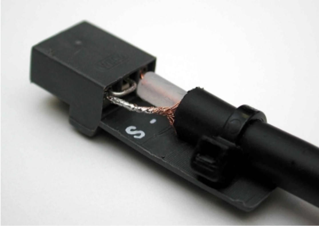
Photo 12 - Coaxial 75-Ohm Unbalanced Digital I/O using WECO HSLConnectors
